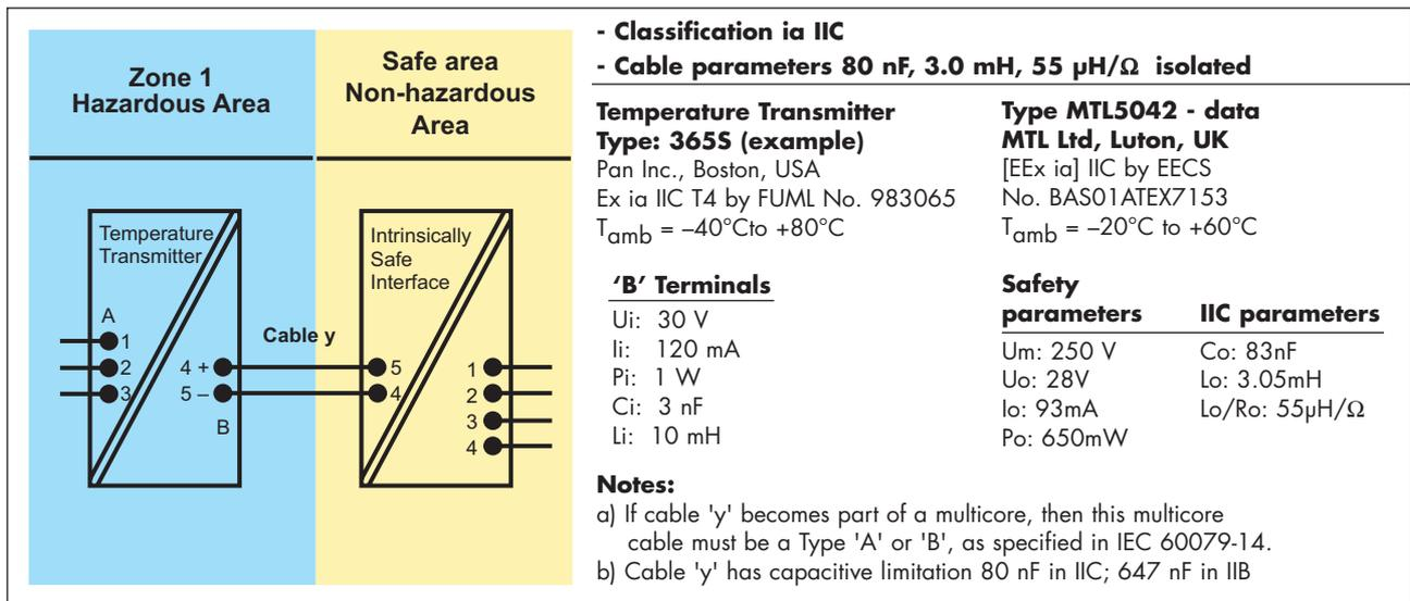
Figure 4.1 Simple system of interface and transmitter
