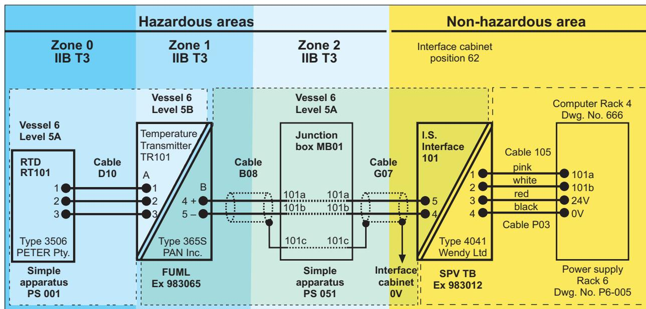
Figure 3.1 - Typical installation drawing for IS system
