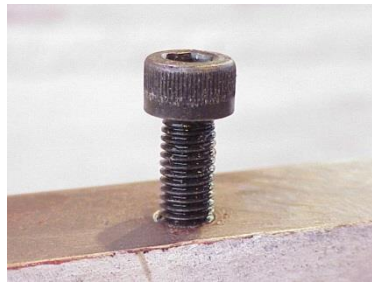
Figure 10: Bolt used in flame proof enclosure
